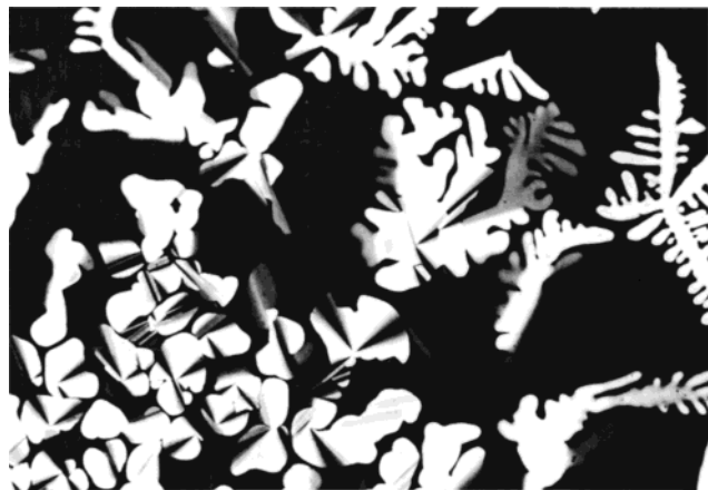
Figure 2. Representative optical micrograph (100 \times ) of texture exhibited by the hexagonal columnar mesophase of P-15-HP at 80 ^{\circ} C on cooling scan.
